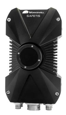
**Workswell SAFETIS Indoor** camera offers great resolution of 640 x 512 px, sensitivity of 50 mK (0.05 °C) and fast response within milliseconds. The powerful communication interface allows connecting SAFETIS camera directly to any computer via Web-server or directly to **SAFETIS Control Unit** via Ethernet RJ45. The SAFETIS camera has integrated 7 digital outputs in the camera and 7 digital outputs in **SAFETIS Control Unit** that can be triggered at the same time if needed.
